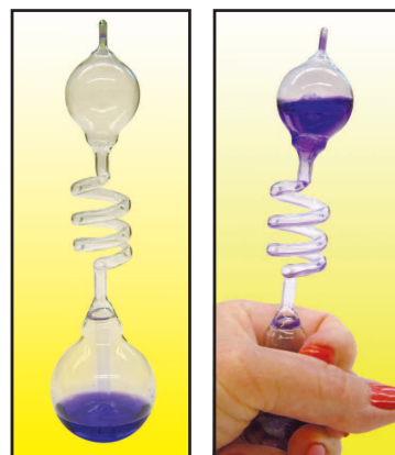
Figure 5. Hand “boiler”. Warming the lower bulb increases pressure, forcing liquid (and eventually vapor) into the upper bulb.
