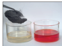
Red drink mix (right) turns colorless after combining with steel wool (left).
